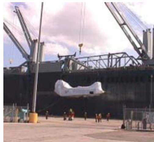
A shrink-wrapped CH-47 Chinook helicopter from the 101st Airborne Division is lifted aboard a large, medium-speed, roll on/roll off carrier at the Port of Jacksonville in preparation for shipment to the Persian Gulf region.
