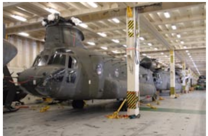
Chinook stowage prior to modification of a deck on the Jean Anne that permits easier transportation of the helicopters
